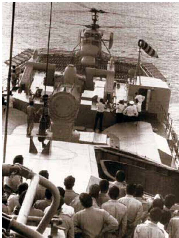
Helicopter landing on a small ship deck is a tricky affair as the pilot must coordinate with roll and pitch of the ship, whilst touching down. Photo: INS Rajput
